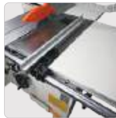
Rip Fence Assembly (Parallel Guide)
