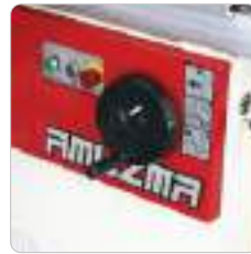
Spindle Height Handwheel and Main Control Panel
