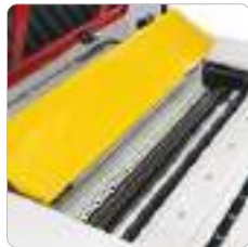
Hinged Internal Chip Deflector
