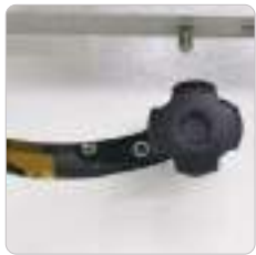
Scoring Blade Adjustment Knob
