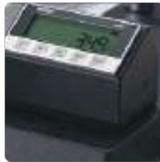
Digital Readout (DRO) for Rip Fence
