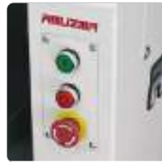
Main Control Panel with Emergency Stop
