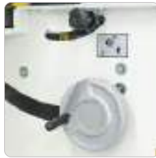
Manual Handwheel for Blade Tilt
