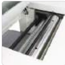
Planer Cutterhead, Power Feed Roller Assembly
