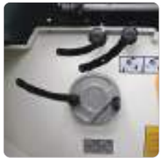
Scoring Blade Adjustment Controls
