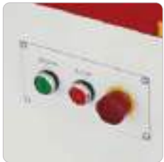
Main Control Panel with Emergency Stop
