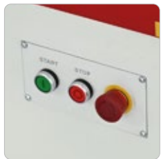
Main Control Panel with Emergency Stop
