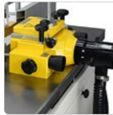
Moulder Fence Hood with Dust Extraction Port
