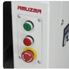
Main Control Panel with Emergency Stop
