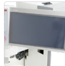
PLC Touchscreen Control Panel
